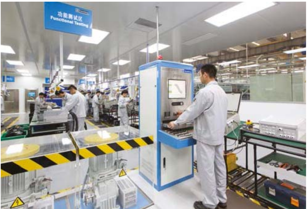
Controller assembly with functional testing
